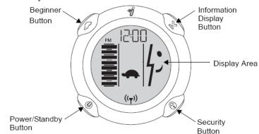
Beginner Button- allows switching from beginner mode (6 mph) to normal mode (12.5 mph), also allows illuminating the backlight.
